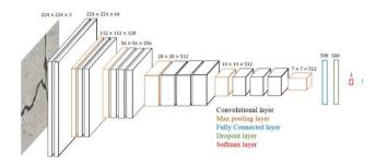
Fig. 1. Architecture of VGG16
